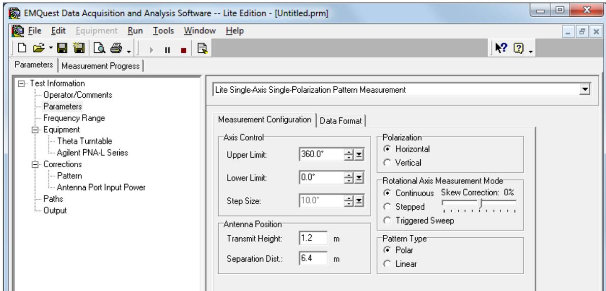
Figure 3. Parameters setup - Measurement configuration (STEP 5).
