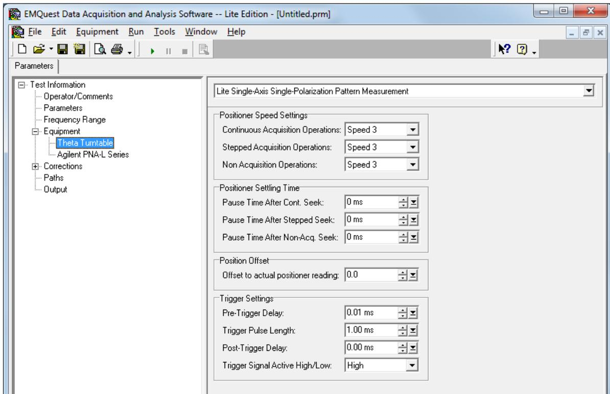
Figure 7. Settings for the theta turntable (STEP 8).
