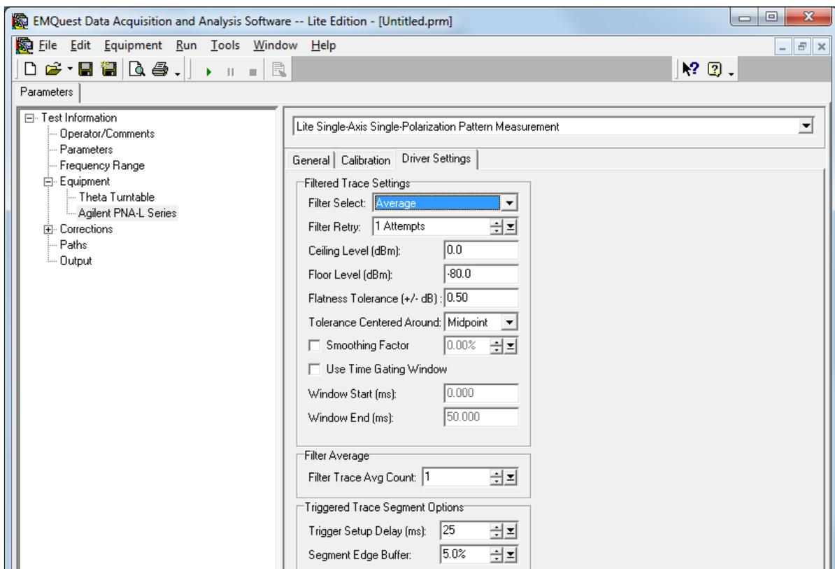
Figure 10. Agilent PNA-L Series driver settings tab.
